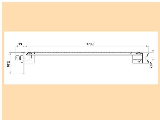
Picture 3 Dimensions plug-in module
