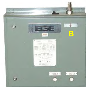
Fig.10 Motor drive MD 3 – control cabinet B.....mechanical indicator
