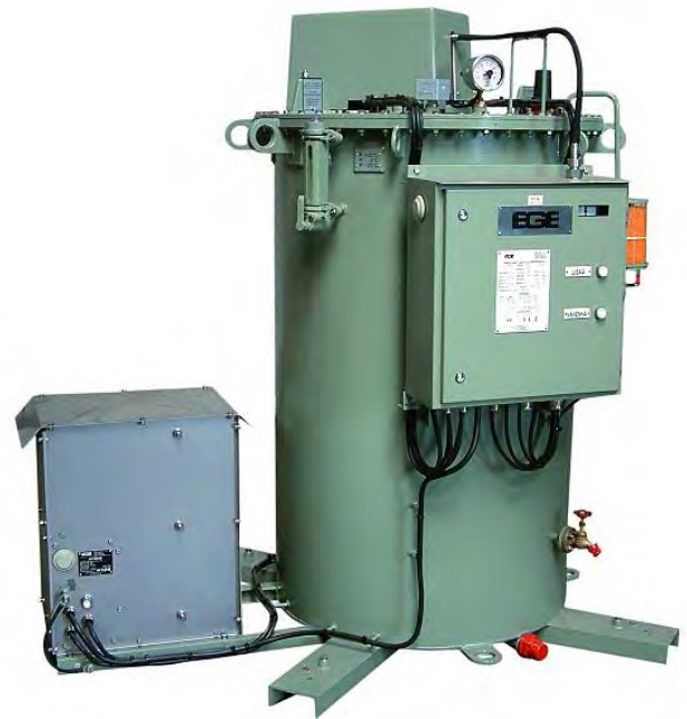
Fig. 4 arc suppression coil - short time duty – without expansion tank (air cushion between transformer oil top level and ASC cover)
