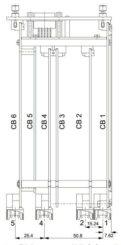
Position of blade connectors and PCBs for feature C00  $\,$
