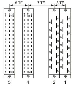
Position of socket connectors for feature C00
