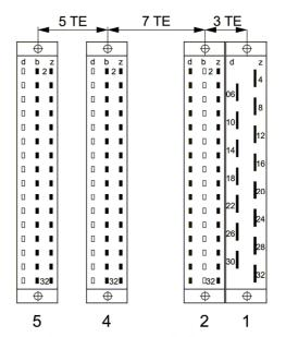
Position of the socket connectors for feature C20... C31
