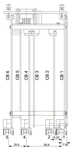
Position of the blade connectors and PCBs for feature C40...C41  $\,$
