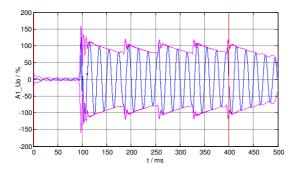
Figure 3:  $u_0(t)$  with a restriking fault
