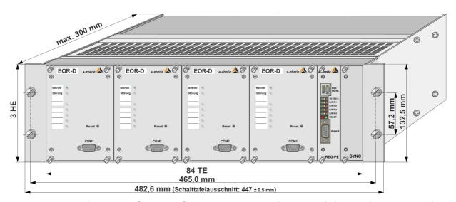
Figure 12: 84 TE rack containing four EOR-D for monitoring 16 control outputs including serial connection to the control (REG-PE)
