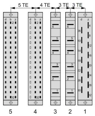
Figure 11: Position of the EOR-D female connectors
