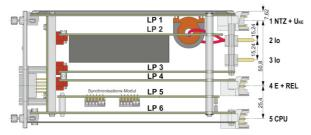
Figure 10: Position of the EOR-D male connectors
