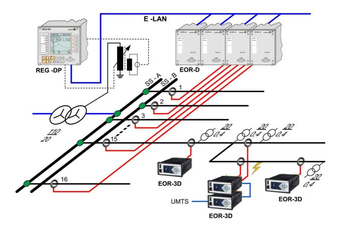
Figure 4: Configuration example for the EOR-D in the substation and the individual EOR-3D devices
