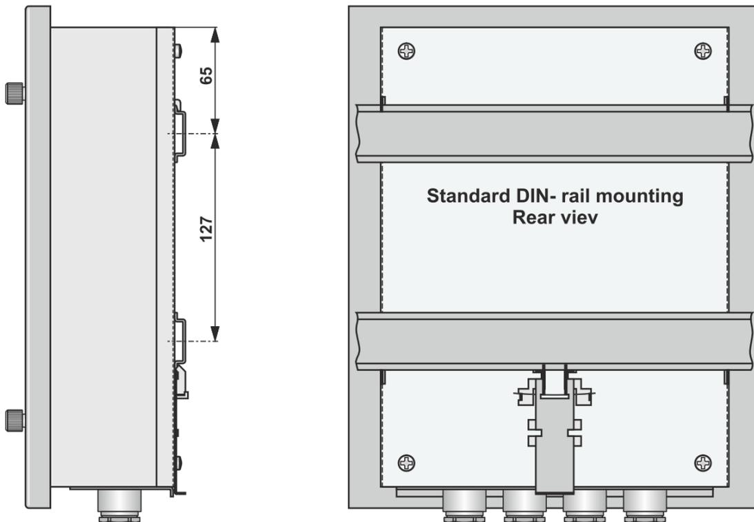
Figure 15: Mechanical dimensions, standard DIN-rail assembling
