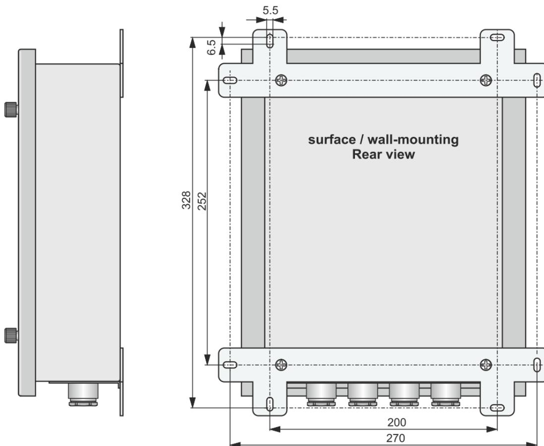
Figure 16: Mechanical dimensions, wall-mounting version
