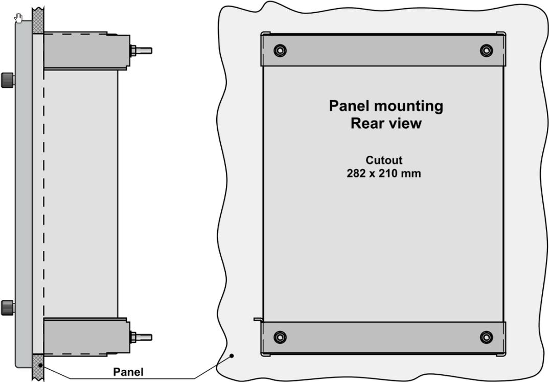
Figure 14: Mechanical dimensions, Panel mount housing
