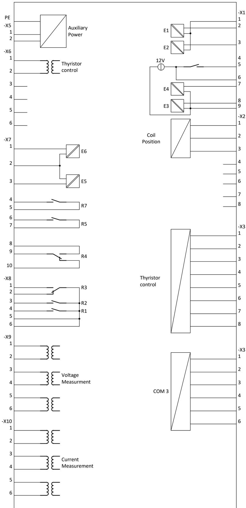
Figure 26: Terminal connections CCI
