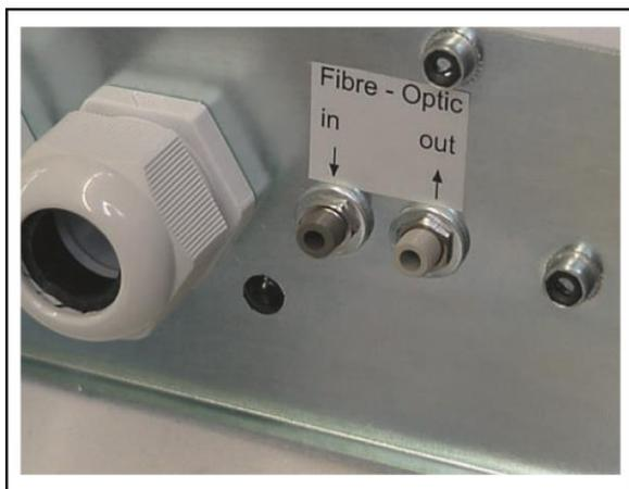
Figure 10: Fibre optic (FSMA-connection)
