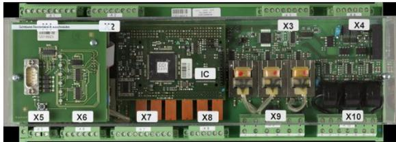
Figure 19: Current feed-in controller (CCI Controller)
