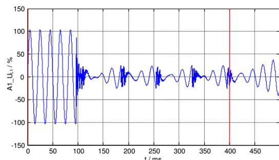
Figure 2: Voltage of the faulty conductor
