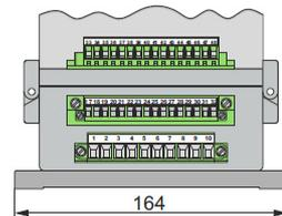
Figure 14: Wall-mounting housing 20 TE
