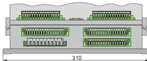
Figure 15: Wall-mounting housing 30 TE with 1 x EOR-D and 1 x BIN-D
