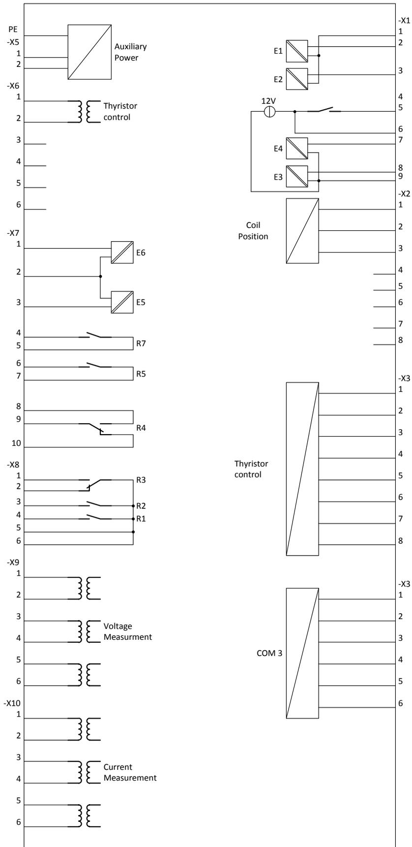
Figure 26: Terminal connections CCI
