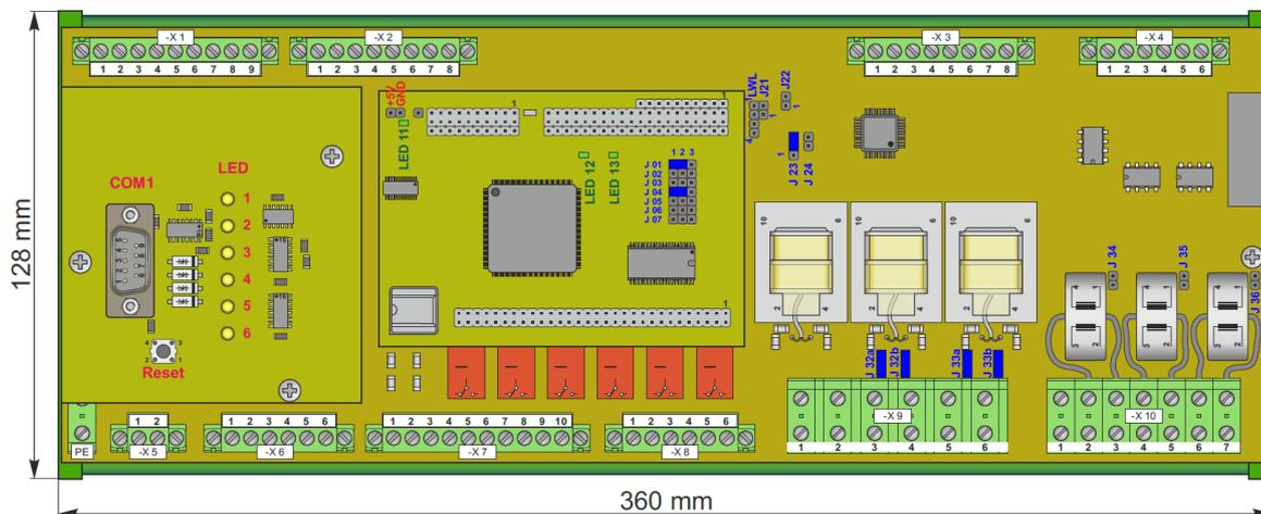
Figure 25: Dimensions of current feed-in controller (CCI)
