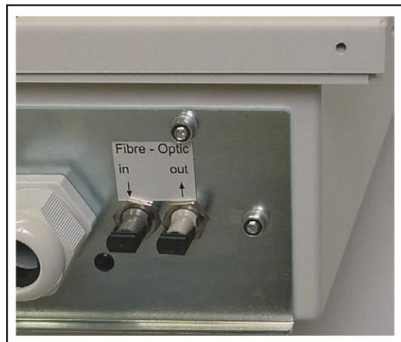
Figure 9: Fiber optic (ST-connection)
