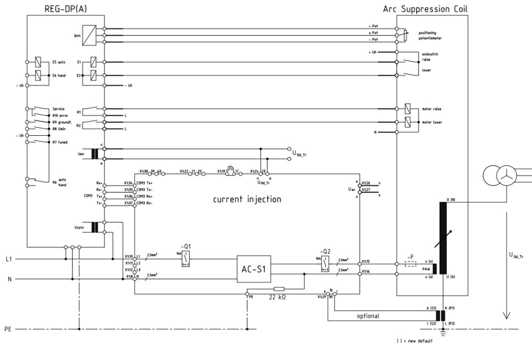
Figure 21: REG-DPA connection, current injection and Petersen coil;
