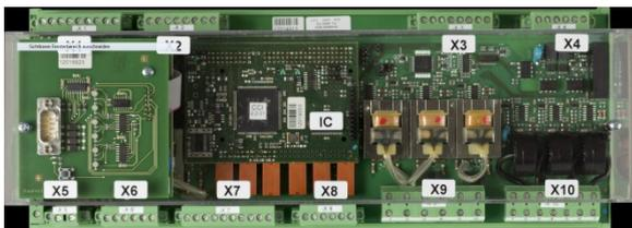
Figure 19: Current feed-in controller (CCI Controller)
