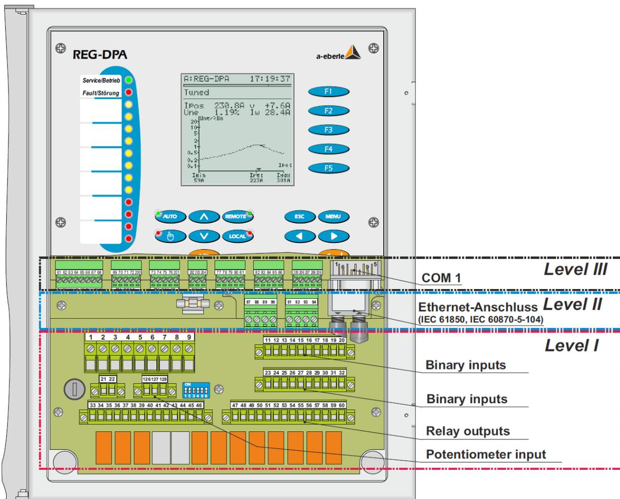
Figure 11: Location of the connector terminals
