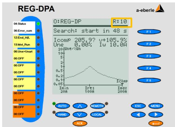
Figure 6: R:10 = Number of possible resistor cycles
