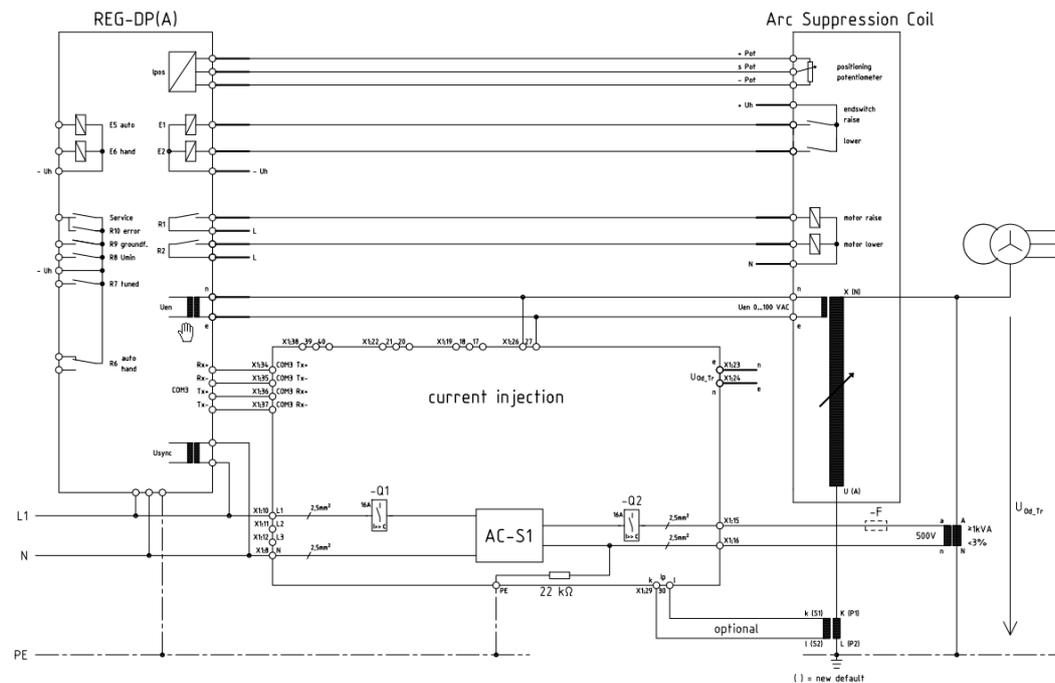
Figure 23: External power auxiliary winding and use of internal voltage transducer for the Petersen coil
