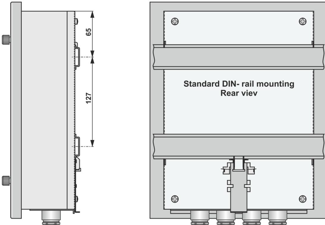
Figure 15: Mechanical dimensions, standard DIN-rail assembling
