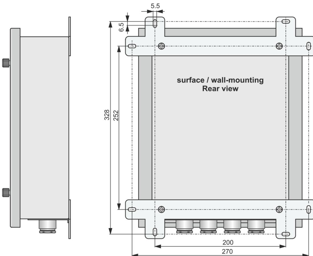
Figure 16: Mechanical dimensions, wall-mounting version
