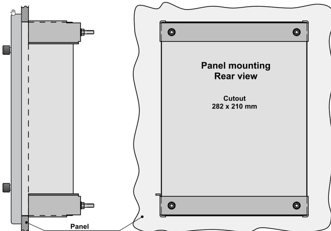
Figure 14: Mechanical dimensions, Panel mount housing
