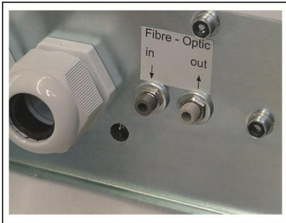
Figure 10: Fibre optic (FSMA-connection)
