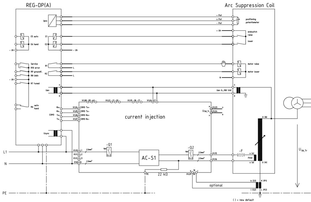
Figure 22:  $U_o$  measurement over external or remote voltage transducer
