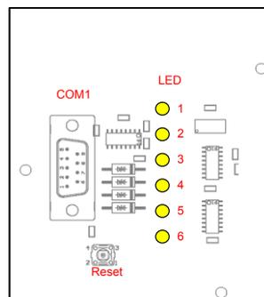
Figure 27: LED definitions current injection controller CCI
