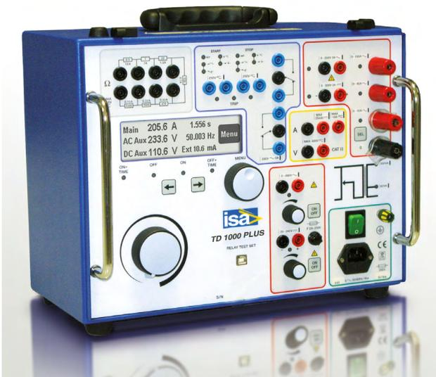
TD 1000 Plus has two current outputs to test differential relay characteristic curve and not only the pick-up current. In addition, the frequency of this current can be changed as with voltages: this allows to test the second harmonic restraint characteristic of the differential relay. Last, the steady voltage output power is increased from 30 VA to 50 VA.
